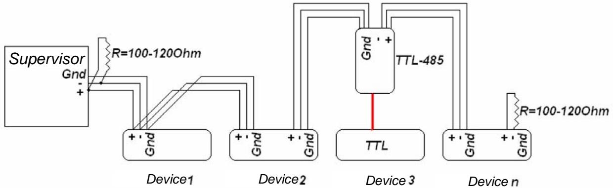
The examples below show networks that are not connected with “daisy chain” layout. All the connection tests will result in communication errors.
