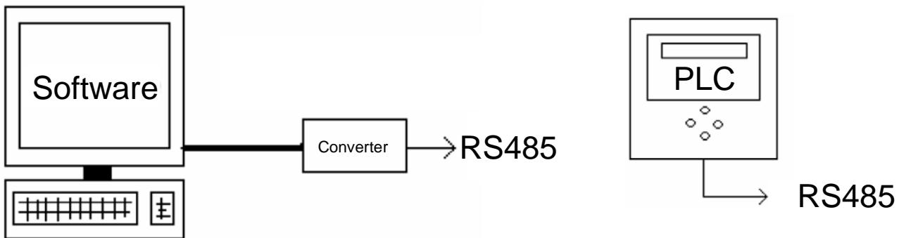
The network must be wired by following the “daisy chain” principle (connection in series without any junction). Prescriptions below should be followed:
