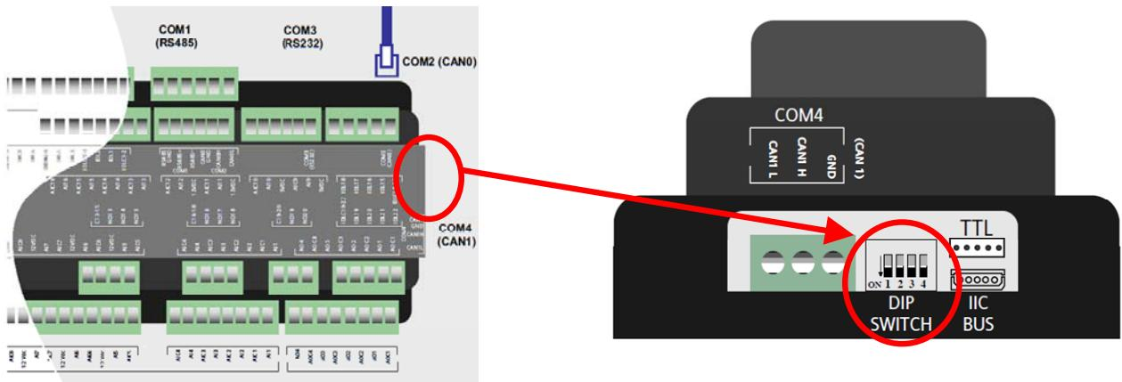
As previously mentioned, the hardware address is made of four bits even though there are only three dipsw. This means the fourth bit is always zero and cannot be changed. As a result, only the combinations within the range of zero and seven are available, while addresses between eight and fifteen are missing.
